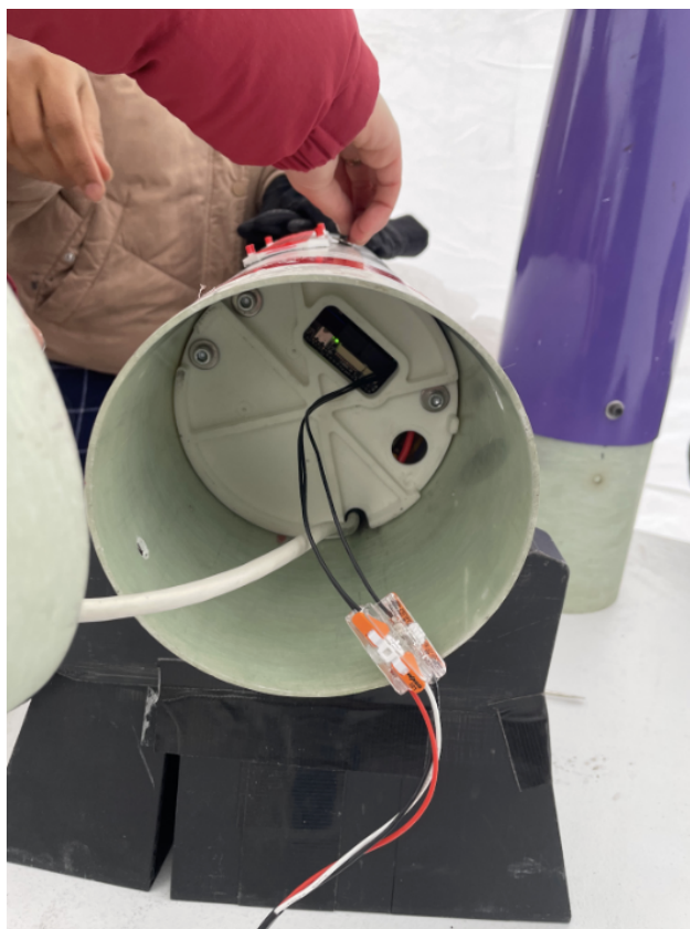
Figure 4: BLiMS installed in the L3 air frame, from below. The green LED visible through the bottom slot indicates the status of the system. The umbilical (white) containing all BLiMS power and control signals runs through its designated port.
