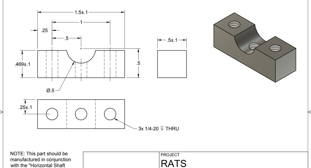
manufactured in conjunction with the "Horizontal Shaft Upper Mount". They should be machined from the same piece of  $\frac{1}{2}$ " aluminum bar, then cut in half with a  $\frac{1}{8}$ " blade yielding the top and bottom components.
